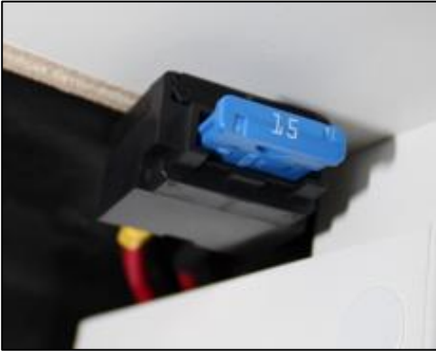
Additional fuse holder, refrigerator (sample illustration)
