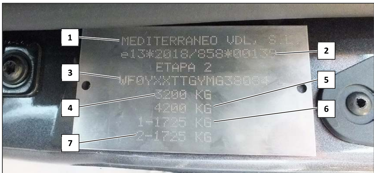
Identification plate in the entry area of the side door (sample illustration)
