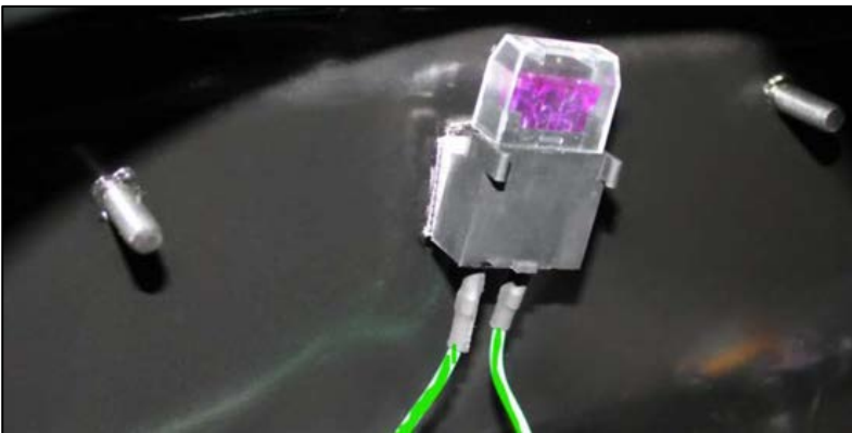
Additional fuse holder for the D+ signal (sample illustration)
