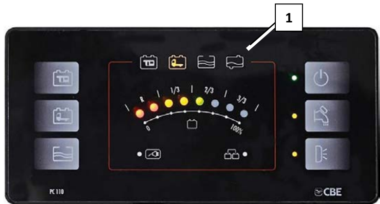
Warning signal for the waste water tank
