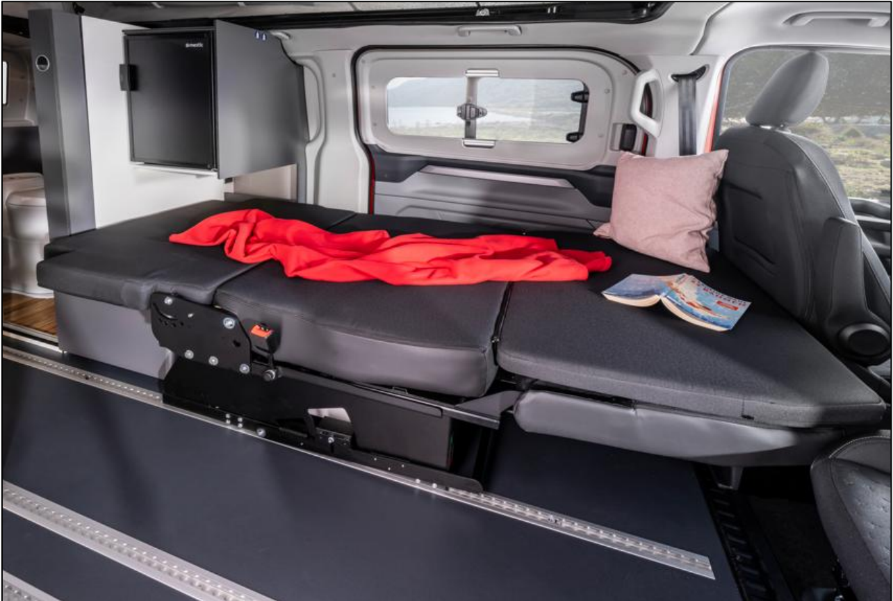
Variable rear bench seat in the DU 550 in sleeping position (sample illustration)
