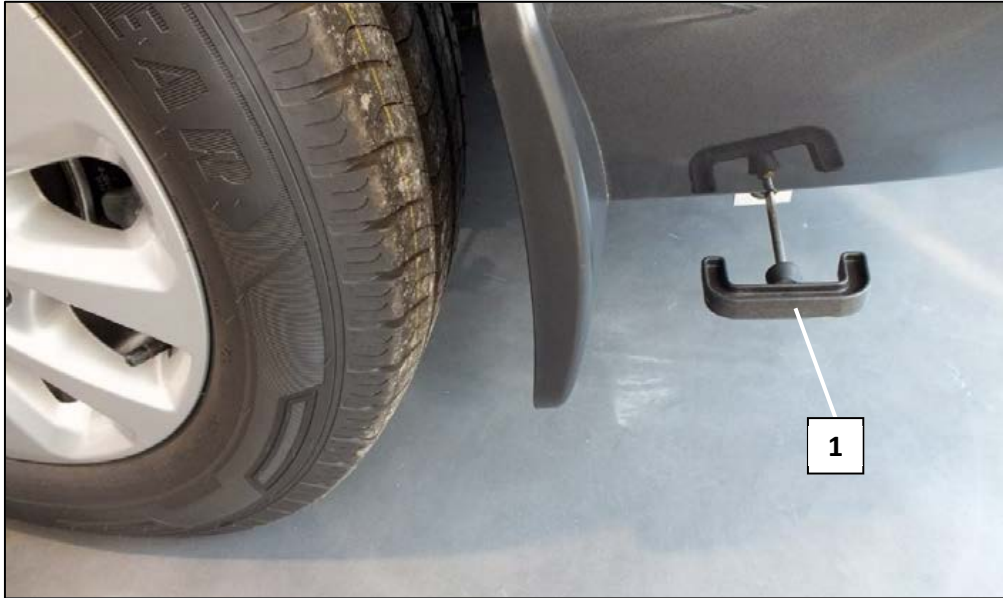
Handle for draining the waste water tank on the DU 550 (open position)
