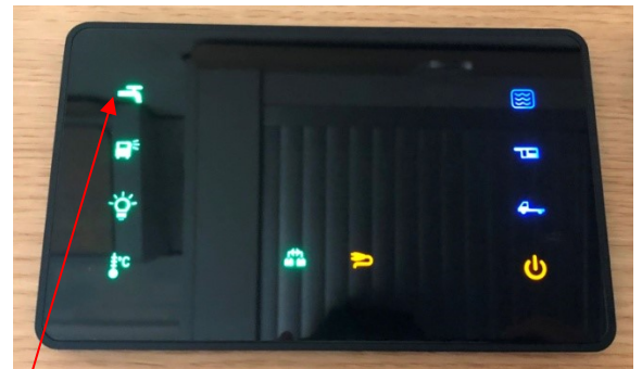
Control button to switch on the electric power supply for the pump
