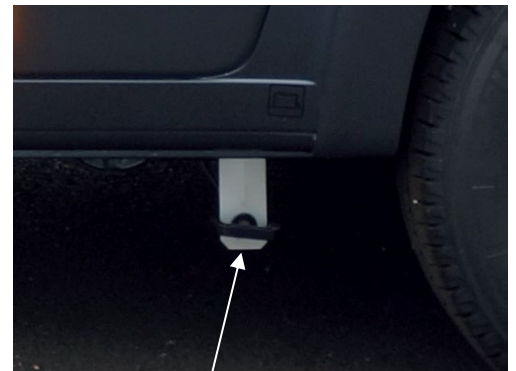
Handle to drain the waste water tank
