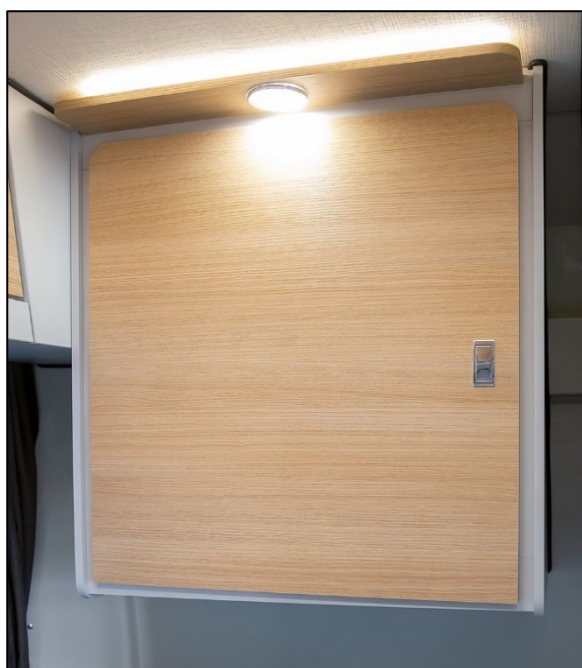
Round spotlight and indirect lighting strip
