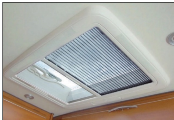
Blackout blind on the roof light
