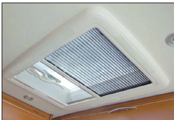
Insect screen on the roof light
