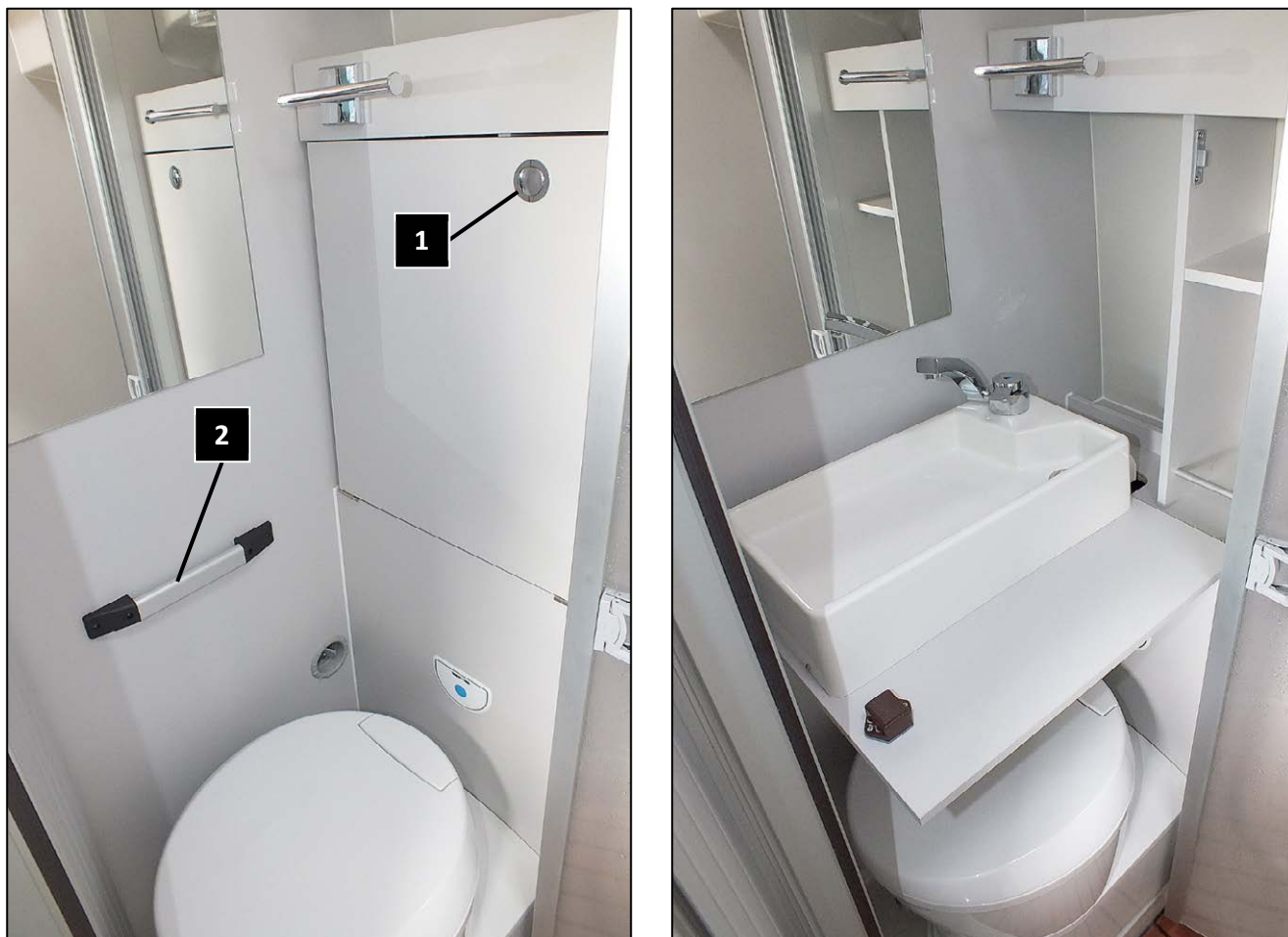
Folding wash basin in the bathroom/toilet. Left: folded up, right: operating position (sample illustration)
