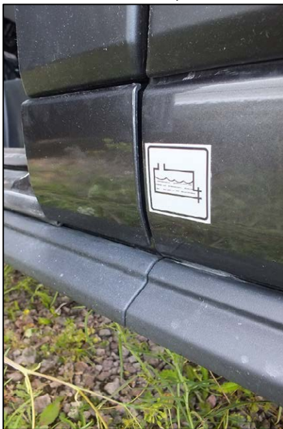
Label indicating the drain valve for the waste water tank (sample illustration)
