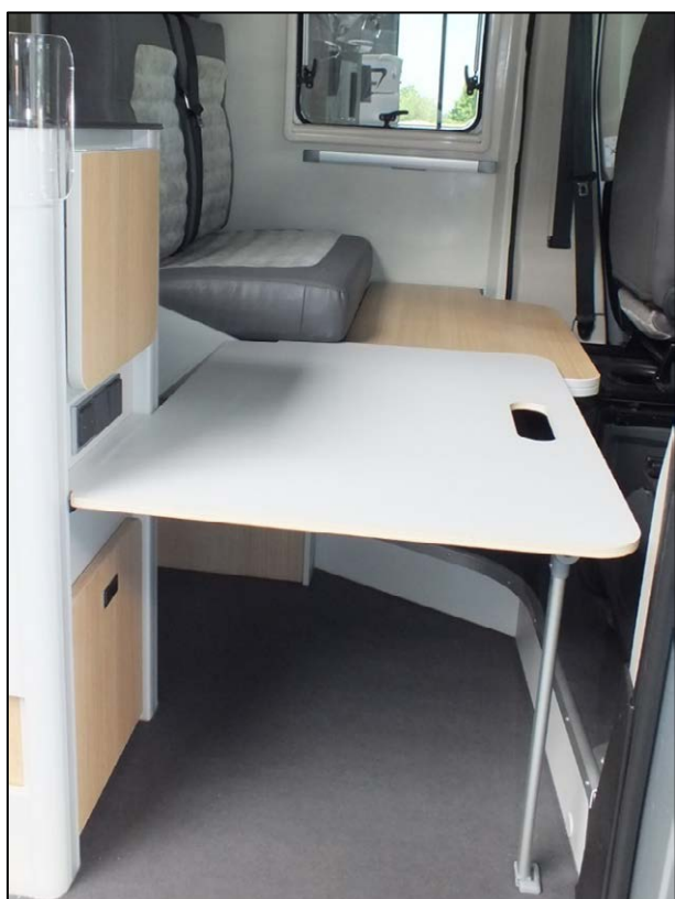
Additional table top attached on the left and supported at the rear*
