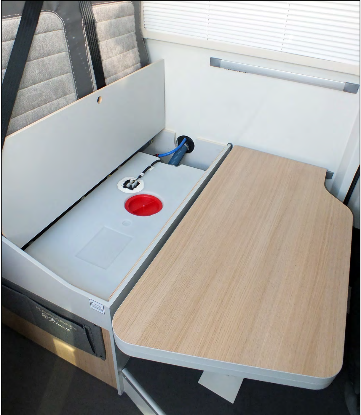
Fresh water tank in the seat compartment of the bench (sample illustration)
