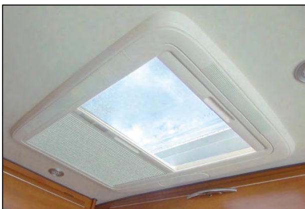
Blind on the roof light
