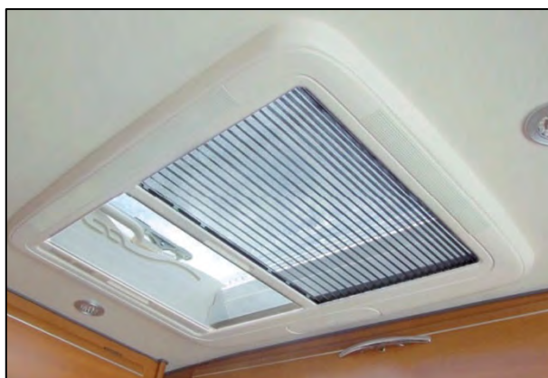
Insect screen on the roof light
