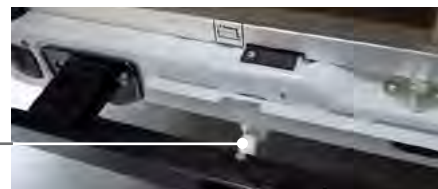
Handle to drain the waste water tank
