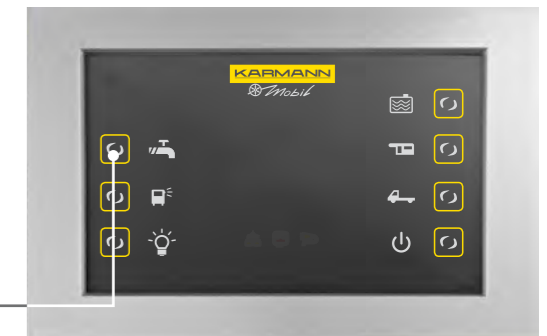
Control button to switch on the electric power supply for the pump
