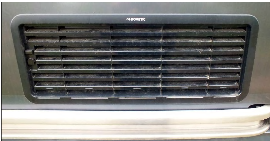
Ventilation opening for the refrigerator on the outside of the vehicle (sample illustration)
