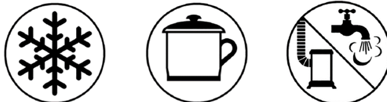
Symbols on the gas shut-off valves, from left to right: refrigerator, hob, boiler
