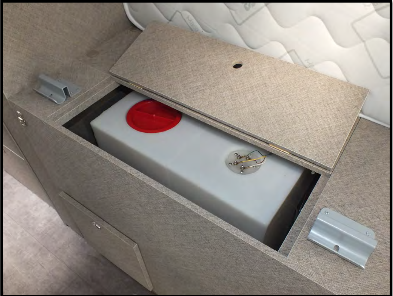
Access to the fresh water tank in the DA 540 TS (sample illustration)
