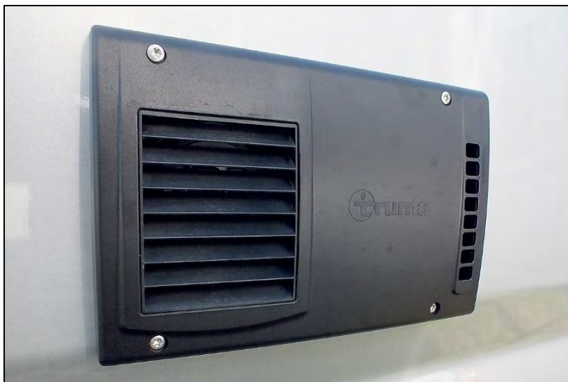
Air intake/outlet element on the outside of Davis LS vehicles (sample illustration)
