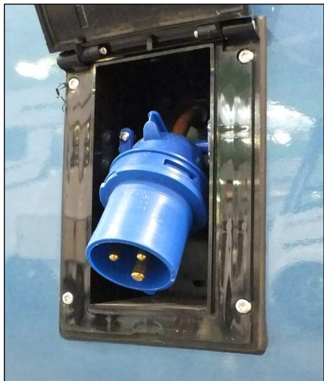
CEE power supply connector (230 V) on the outside of the vehicle (sample illustration)
