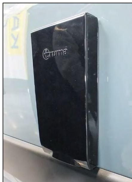
Air intake/outlet element of the boiler on the outside of the Davis with TS specification (sample illustration)
