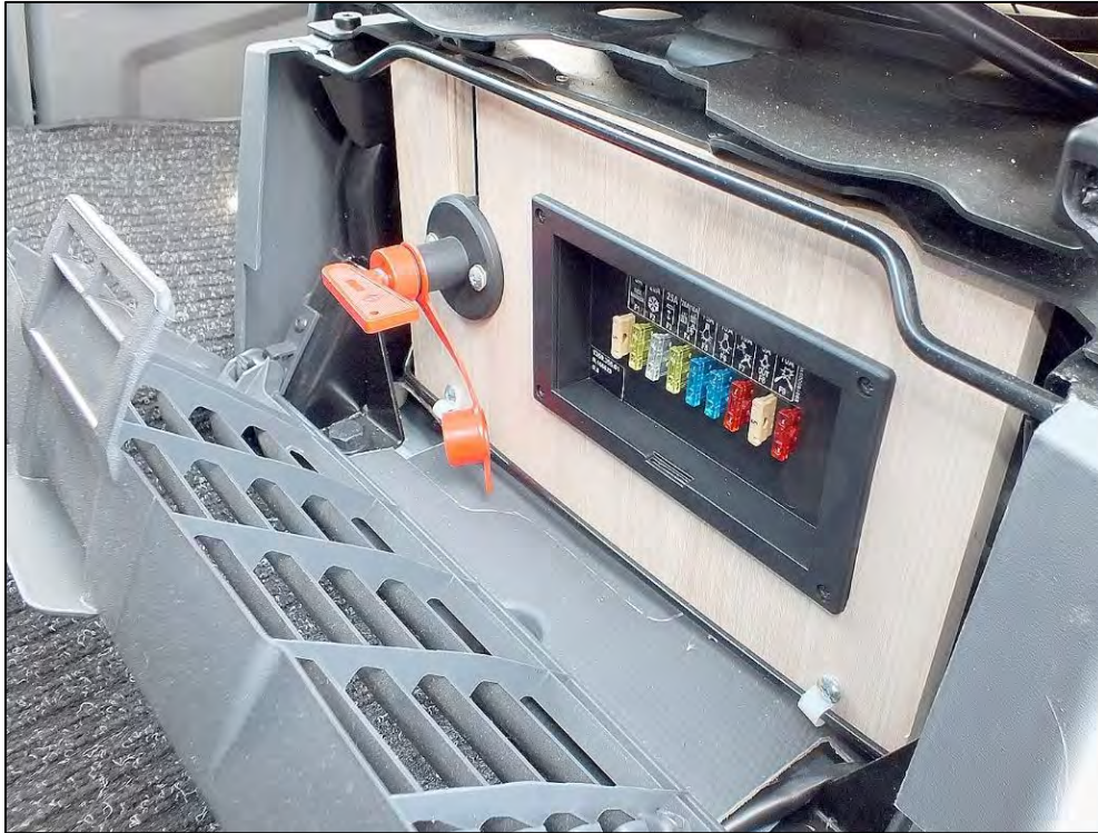
12 V fuse box with distribution function and battery disconnect switch (sample illustration)
