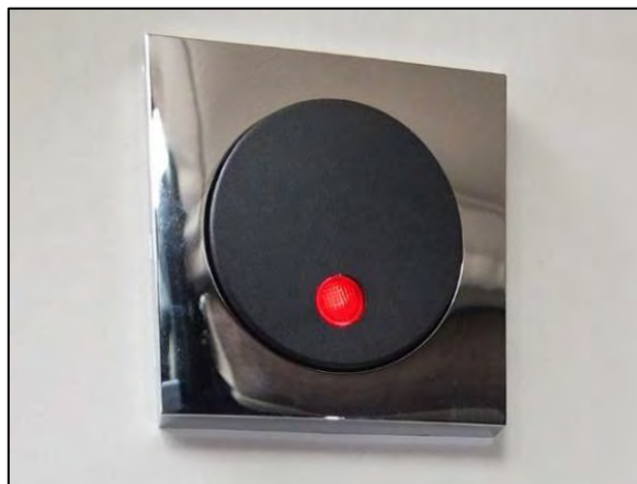
Switch for waste water tank heating, “On” position (sample illustration)
