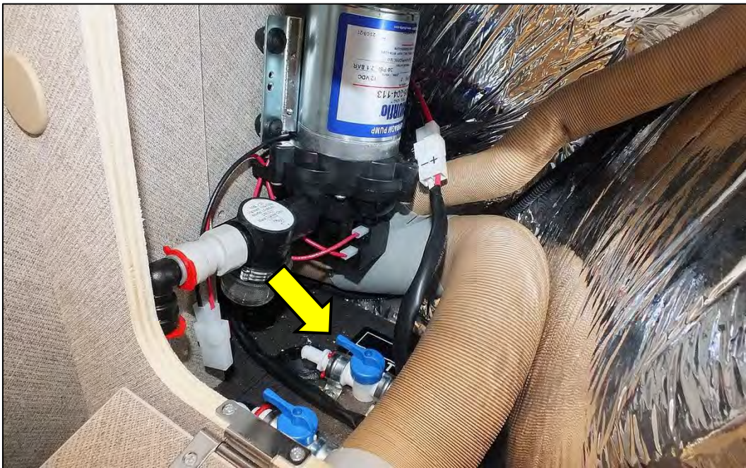
Drain valve "drain fresh water tank to 20 l" in the DA 590/ 591 with 137 l refrigerator (sample illustration)
