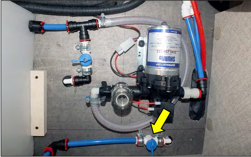
Drain valve "drain fresh water tank to 20 l" in the DA 591 (sample illustration)
