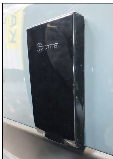
Air intake/outlet element of the boiler on the outside of the Davis with TS specification (sample illustration)
