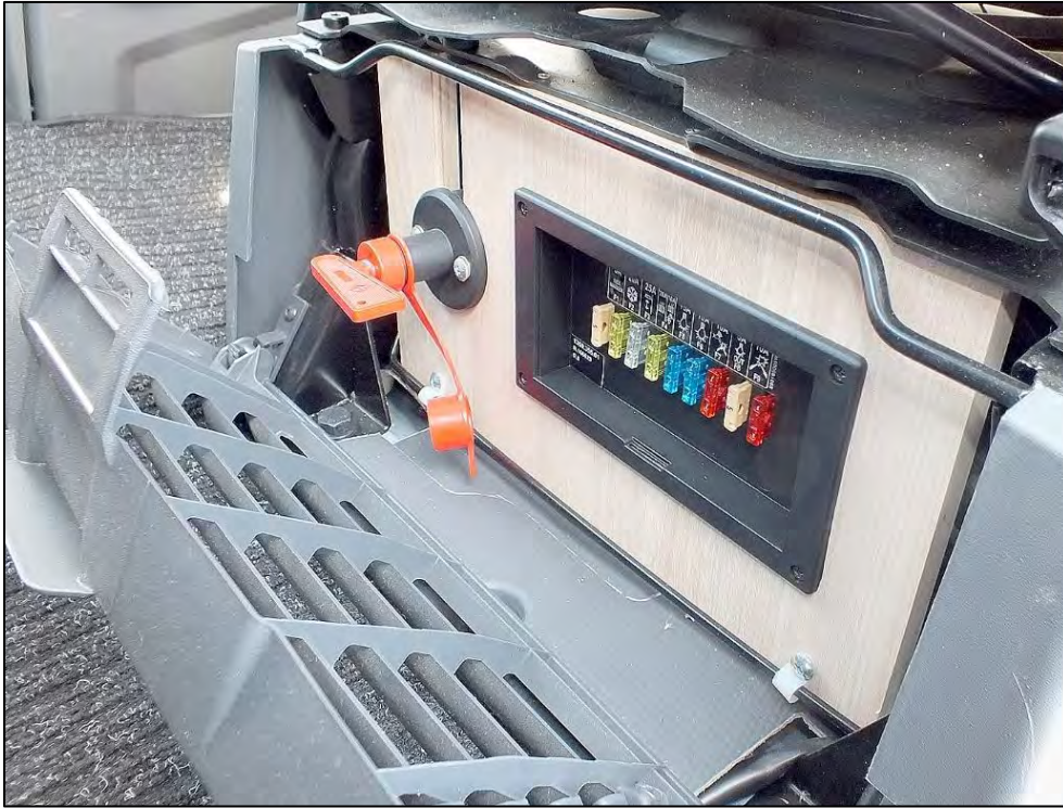
12 V fuse box with distribution function and battery disconnect switch (sample illustration)
