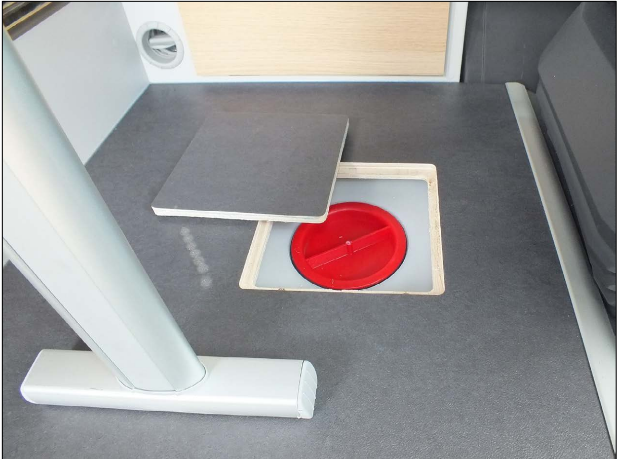
Access to the fresh water tank
