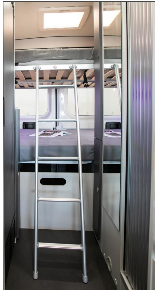
Right: Ladder attached to the slatted base of the raised bed in the Dexter 581 (sample illustration)
