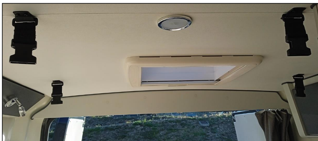
Buckles on the vehicle ceiling for attaching the safety nets of the raised bed (sample illustration)
